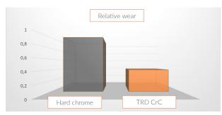
Performance results of an abrasive Micro Wear Test for hard chrome and TRD CrC coatings. The wear performance of TRD CrC is almost tripled compared to hard chrome.
